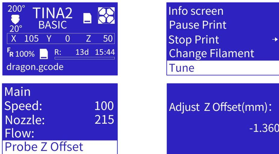
ALLOWS REAL-TIME Z-AXIS ADJUSTMENT TO CHANGE GAP DURING PRINT:
