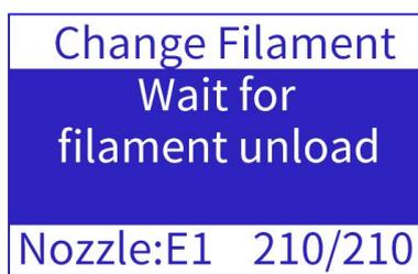
Beep indicates unload complete, insert new filament as prompted and press knob.
