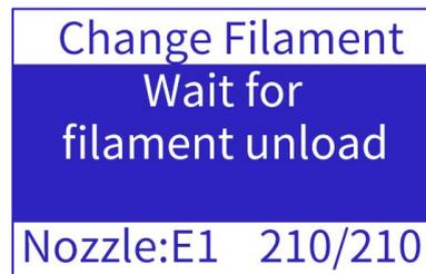
Beep, insert new filament, press knob. Auto-load at temp.
