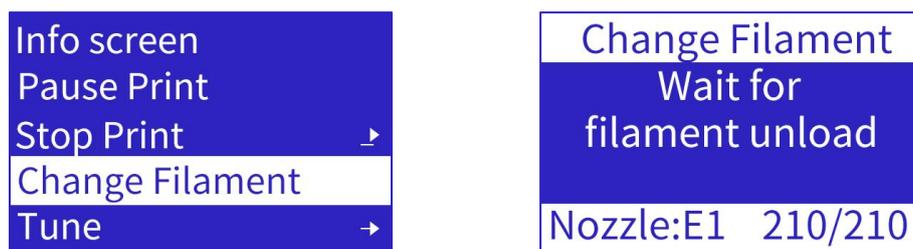
Beep, insert new filament, press knob. Auto-load at temp.
