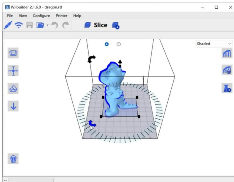
Model should be centered and properly placed on platform. Click Center Object, Flat, Land Object. If floating, print fails.
