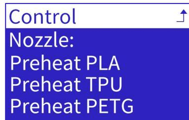
Select Nozzle, turn knob to desired temp, press to confirm.
