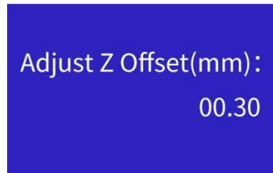
Turn knob to precisely adjust nozzle height for smooth, flat first layer.
