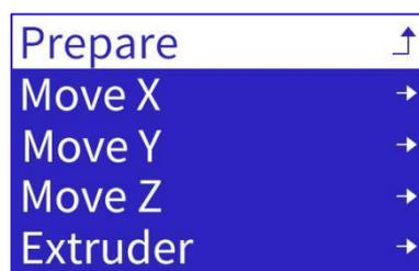
X/Y/Z Axis: 10mm, 1mm, 0.1mm increments
